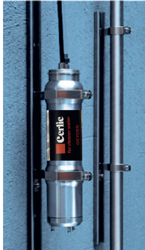
SS Slide rail assembly for easy installation and servicing. Available in two sizes 20 mm Ø for pH, ORP and FLX and 66 mm Ø for O2X and TSS sensors. The rail has field adjustable stop. It's easy to install and to inspect sensors for cleaning and calibration.
