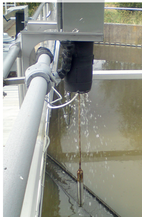
The CBX is built into a stainless steel enclosure for installation in a variety of environments. It has automatic flushing of both sensor and cable after each soldering.
