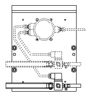
Mounting plate P/N 10305533 for one or two solenoids, outside US version P/N 11705516A (11705516 B US Version) and a connection box P/N 11505748.
