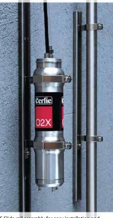
SS Slide rail assembly for easy installation and servicing. Available in two sizes 20 mm Ø for pHX, ReX and FLX and 66 mm Ø for O2X and ITX sensors. The rail has field adjustable stop. It's easy to install and to inspect sensors for cleaning and calibration.
