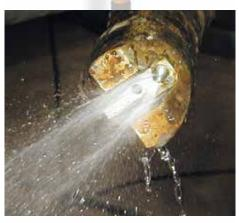
The automatic flushing device has no moving parts and ensures minimal maintenance and enhanced reliability. The flushing nozzle uses water or compressed air.
