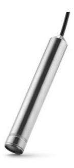
Level transmitter with submersible probe in stainless steel for level measurement in vessels where pressure connection in the bottom of the vessel is not possible or desirable. For exampel pump pits, reservoirs or plastic tanks.
