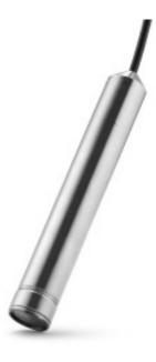
Level transmitter with submersible probe in stainless steel for level measurement in vessels where pressure connection in the bottom of the vessel is not possible or desirable. For exampel pump pits, reservoirs or plastic tanks.
