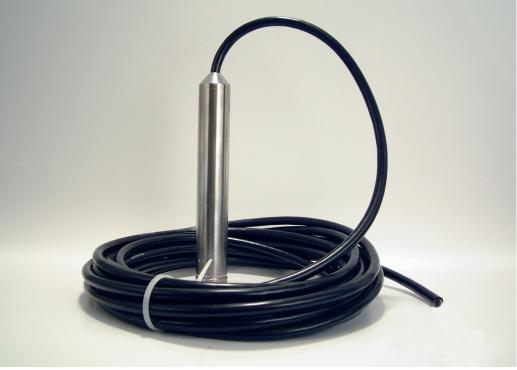
Level transmitter with submersible probe in stainless steel for level measurement in vesselswhere pressure connection in the bottom of the vessel is not possible or desirable. For examplepump pits, reservoirs or plastic tanks.
