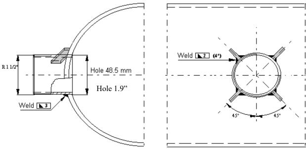
Mounting of weld end with strip iron
