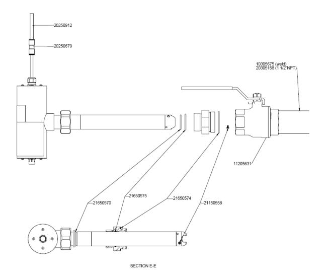
Nipple 10305675 is to be cut to make the bottom of the measure gap be at least 5 mm  $(\frac{1}{4})$  from the pipe wall.
