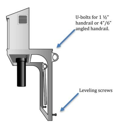
Mount the CBX so there is no risk that the sensor will be stuck in something on the way down in the basin. This is extra important for outdoor installations where wind can make the sensor swing so much that it is a risk that it will stuck in, for example a hand railing.
