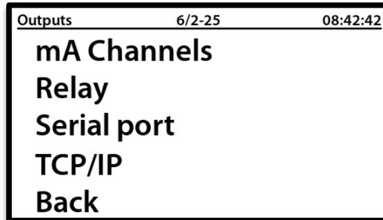
There is support for two different serial ports on the C-tron. Partly a standard RS485 and a ModBus RTU. Press on
