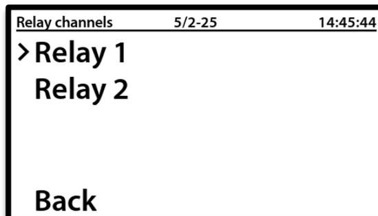
With this function, you can activate the relay that will control the cleaning flush of the sensor. Press on
