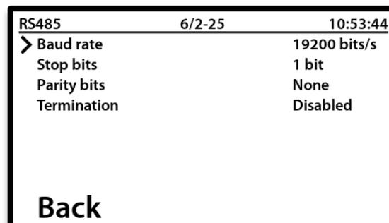
Then step by pressing
