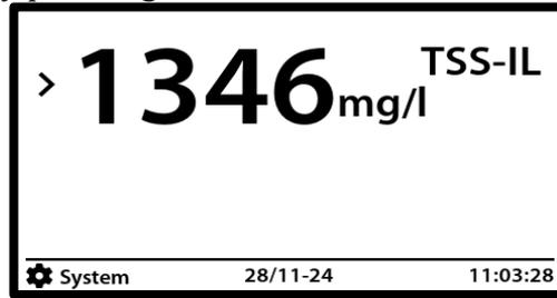
Go to Reset Sensor by pressing
