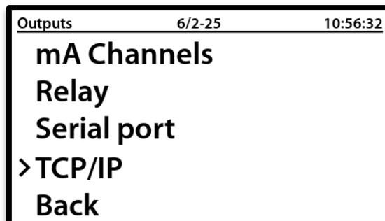
There is support for two different TCP/IP ports on the C-tron, Ethernet and a ModBus TCP. Press on
