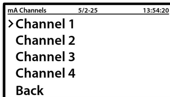
In this menu you can select the source for mA output 1. Default is sensor i connected to mA output 1. Sensor 2 connected to mA output 2, etc. Press on
