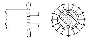
Fig. 2 Connection of the shield braid to the washer
