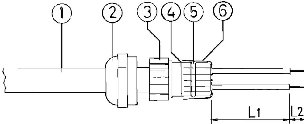
**Fig. 1 Cable with shield and screw connector.**
