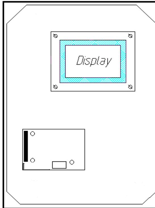
Mounting the module in the control box
