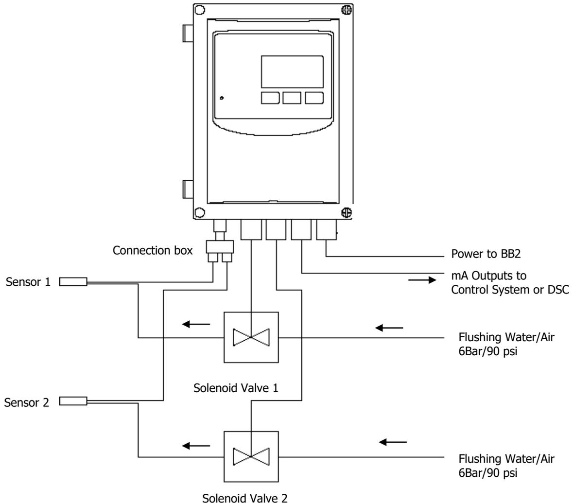
**Figure 1** Connection of BB2 Control box with two sensors and two flushing valves
