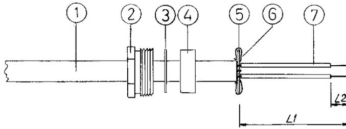
**Fig. 1 Cable with screw-on parts**
